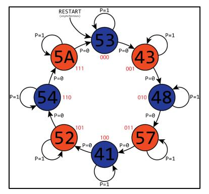
So here I called the output number "53" state 000, the output number "43" state 001 and so on. You can technically use any number you want for the given states, but it is usually much easier to just use the numbers 000, 001, 010 and so on. Now that the states have been given values, we know how many and which FFs to use, as well as how many outputs we need, it's time to make the table!
