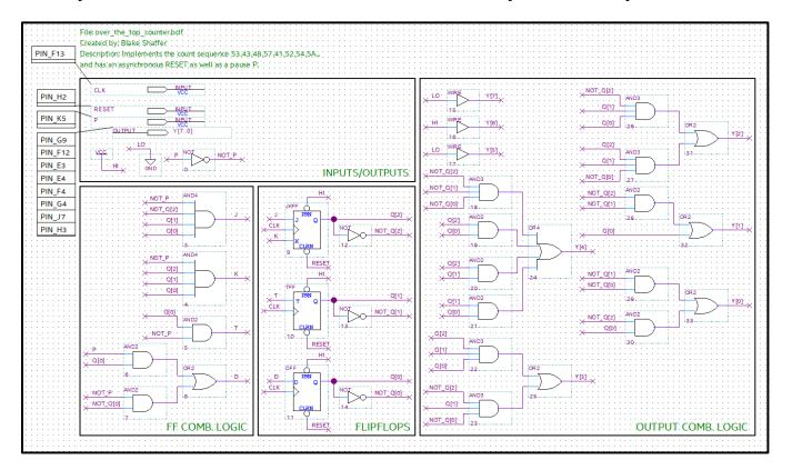
This bdf has the required flip flops in the middle, the combinational logic for all the flip flops on the left side and the combinational logic for all the outputs on the right.
